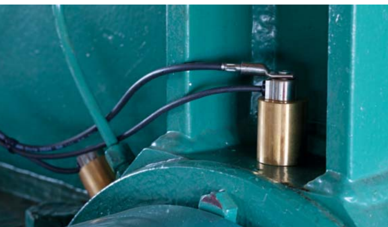
Two vibration sensors each, installed slightly shifted, permanently monitor the condition of the rotating bearings.
