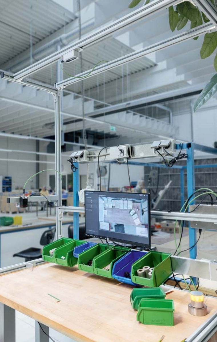
ifm mate as a complete solution: Camera (above the workstation), software and PC can be easily extended with a touch screen, a signal lamp (bottom right) and an O2D5 vision sensor (far left, mounted on crossbar).
