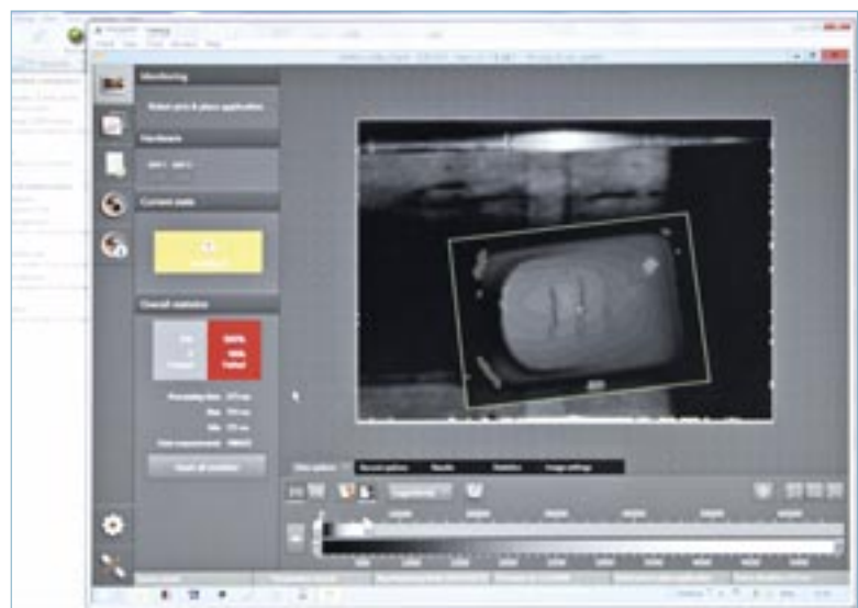
The baggage position can be checked with the ifm Vision Assistant using a 2D image. The camera also provides distance and grey-scale images.
