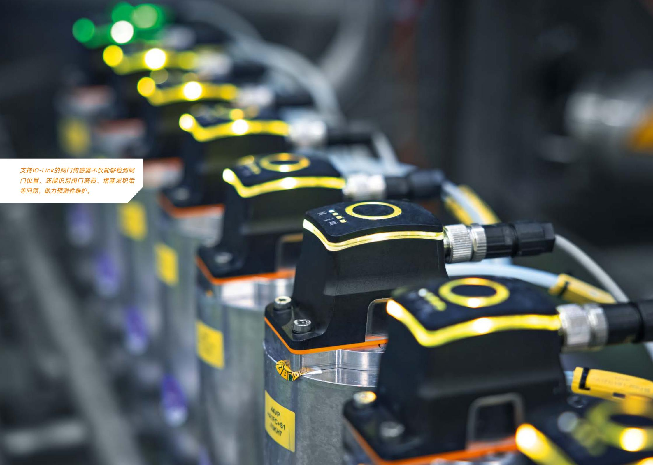
A row of industrial valves with IO-Link sensors in a factory setting. The valves are black and yellow, with yellow cables connected to them. The background is blurred, showing other industrial equipment and lights.
