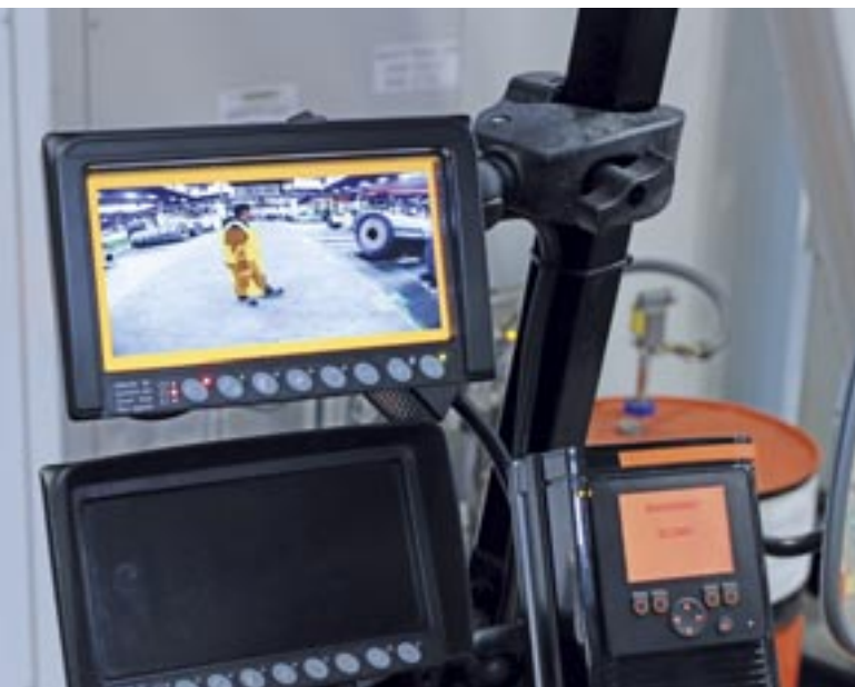
The driver sees the rear area of the forklift truck on the monitor. Colour-graded frames indicate objects in the path and display further warnings up to an e-stop.
