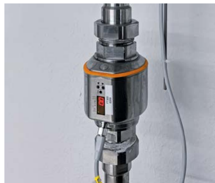
The flow sensor transmits several measured values to the control system via IO-Link.
