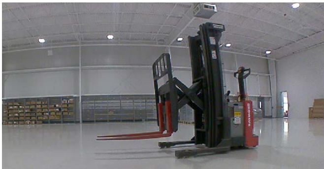
The robotics platform captures the situation in a 2D image and in 3D distance data.
