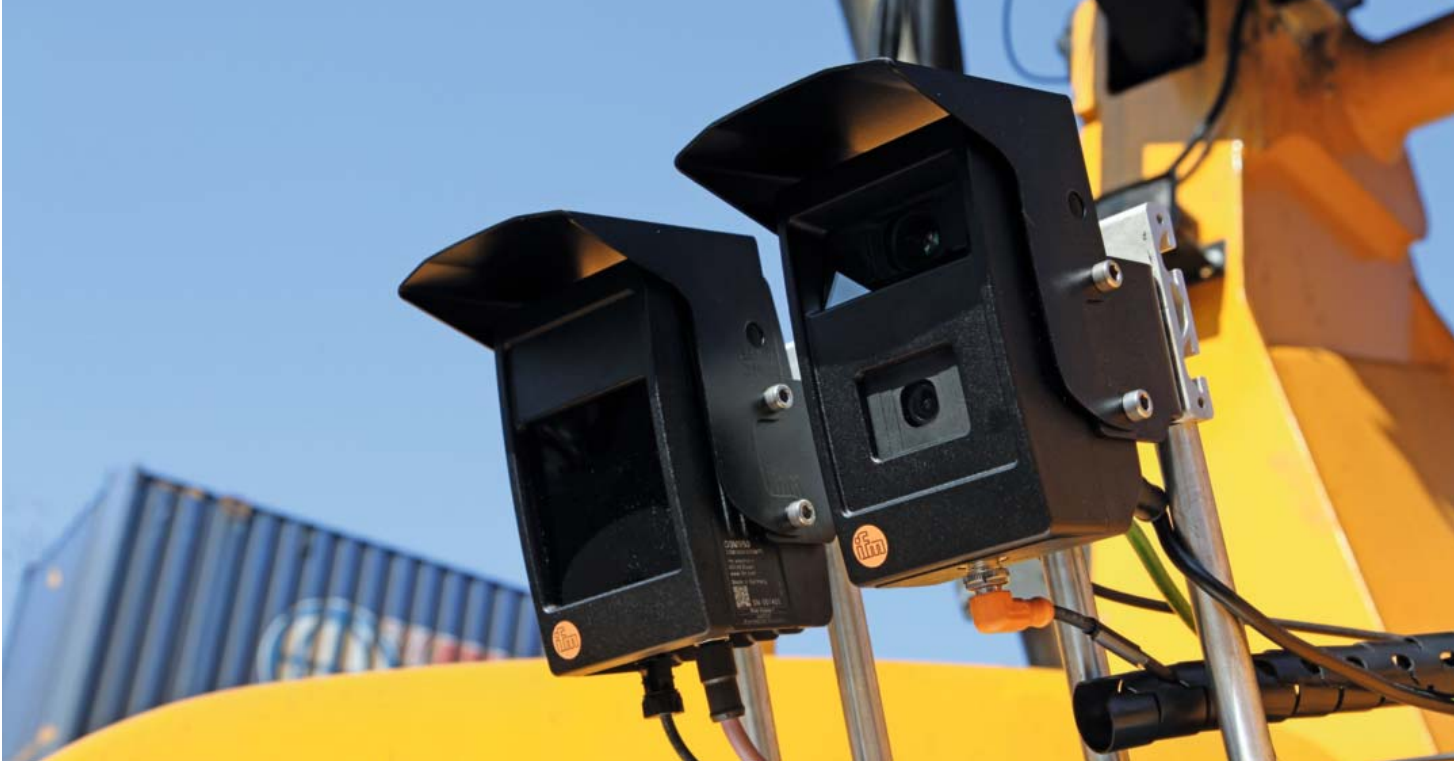
O3M system: 3D camera (right) and infrared illumination unit (left).
